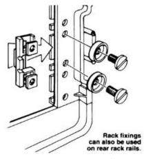
16-785 CP EMS111 SPARE FIXINGS KIT For EMS 400/500 series rack case, (set of 12) EMS111 contains 12 rack bolts, nuts, plastic cup washers and 6 nut holders that accommodate two nuts.
