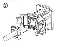
Follow the direction instruction on termination cap and place the termination cap onto the socket properly.
