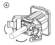
Close the housing firmly, ensuring good connection between earth wire and housing.
