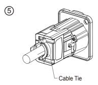
Fasten the cable tie to secure the cable in the socket.
