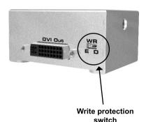
Once the DVI Detective is programmed and working, you can write protect the unit to prevent an accidental overwrite. This is done by simply moving the write protect switch to the D (write disabled) position. By default, the unit is shipped in the E (write enabled) position. This is done so that the unit is ready to be programmed right out of the box. Whenever the unit is going to be programmed, make sure that the switch is in the "E" position, otherwise the procedure will fail.
