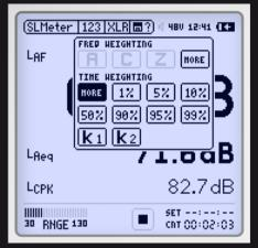
The Extended Acoustic Pack supports the daily tasks of acoustic consultants. It offers additional features for sound level logging and acoustic measurements, such as recording linear wav-files, percentile statistics, sound exposure level, 100 ms logging, event monitoring, RT60 in 1/3 octave resolution, Zoom-FFT with 0.4 Hz resolution and many more.
