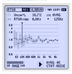
Measure the energy decay with automated triggering using an impulse signal or gated pink noise as signal source, and determine if the room fulfills the RT60 requirements.
