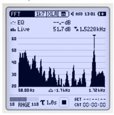
The real-time FFT is the ideal tool for visualization of comb filters and narrow band effects. It measures the actual level and the averaged level Leq in three ranges over the entire audio band.
