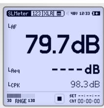
The XL2 provides a precise sound level meter for events and environmental noise monitoring. Numerous measurement variations are simultaneously available. Actual level, Lmin, Lmax, Leq may be measured in combination with frequency weighting A, C or Z and time weightings fast, slow and optional impulse. All results are simultaneously available.
