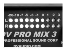
Meters Showing 0dB Signal Level (Signal level O.K., your faders are set correctly)
