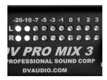
Meters Showing -10dB Signal Level (Signal level too low, correct by raising input fader level)
