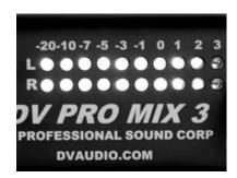
Meters Showing +2dB Signal Level (Signal level too high, correct by lowering input fader level)
