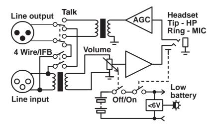
Fig 1-2: CM-BH4W Block Diagram
