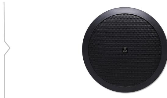
The CM20T two-way built-in loudspeaker can be used as a 16 ohms or 100 volt loudspeaker. In 16 ohms use, you can connect up to 4 loudspeakers in parallel on each channel of a standard 4 ohms amplifier. For 100 volt use, the CM20T is equipped with a high-quality 20 watts 100 volt transformer with several power tappings (20 – 10 – 5 – 2.5 watts). Therefore it can be used in projects with high ceilings or places with background noise where a little more power is needed.
