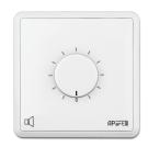
The Apart E-VOL40 is a 100 volt volume control that can handle up to 40 watts of power. It is very versatile thanks to the step-by-step attenuation in 11 steps + zero position. The E-VOL40 is designed to handle 24V priority signals. This means that you can always get an announcement out, even to zones where the local volume control is in the 'OFF' position!
