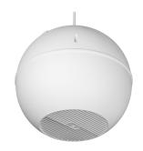
The Apart EN-SPH6T20-W is a 6" sphere loudspeaker with ABS housing (RAL 9016 equivalent), equipped with a high efficiency full range speaker and a multi tap 100 volt transformer, all certified according EN 54-24.
