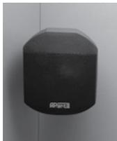
Now slide out the rubber security piece from the back of the speaker, slide the speaker on the H-hook of the mounting bracket. Slide the rubber part back in place to lock and secure the cabinet. Plug the euroblock connector into the speaker.
