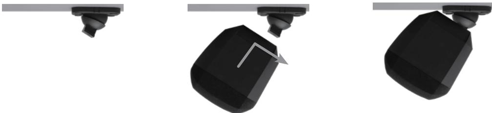
Using the appropriate mounting hardware, mount the bracket to the ceiling. Mounting materials for solid brick walls are included. For other materials you may need other hardware, available from your local hardware store. Slide the speaker onto the mounting bracket in such a way that it won't slide off even without the rubber locking piece in place. After you slide on the speaker, slide the rubber part back in place to lock and secure the cabinet. Plug the euroblock connector into the speaker.
