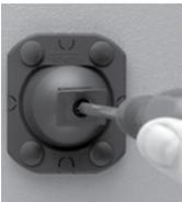
The angle can be determined by the position of the bracket base and the position of the H-hook on the half-sphere ball. The factory default force-setting of this central screw is adjusted for moving the H-hook over the semi-sphere with or without the cabinet being over the hook. It is allowed to adjust the angle by moving the cabinet and the H-hook together after the mounting has been realized. You can fasten or loosen the central screw to influence the turning force of the H-hook.
