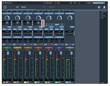
10. Set the "Orientation," "Pattern," and "Tilt" of the virtual microphone for each channel.
