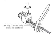
2. Loosen the screws with a flathead screwdriver.
