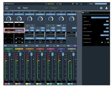
4. Set "Priority", "Can Cut", and "Off Attenuation" for each channel, as necessary.
