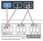
When "Output Flip" is turned on, the OUTPUT ST notation on the audio output screen changes to OUTPUT L/R.
