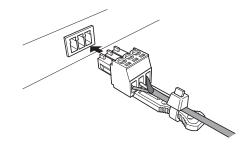
Verify the pin assignments, and connect each to the applicable wire.
