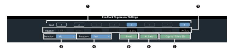
The statuses of the bands appear. It can also switch between dynamic and static.
