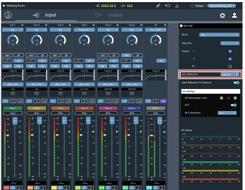
4. Turn AEC ON for the microphone to be used (for each channel).
