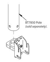
3. TIGHTEN GRUB SCREWS (ITEM 6) TO FIX COLLAR TO POLE
