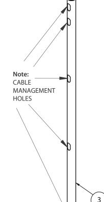
**Note:** Position pole so the cable management holes face the rear of the stand.
