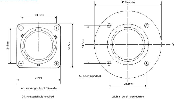
44-854 26 pin panel socket, with bayonet pins
