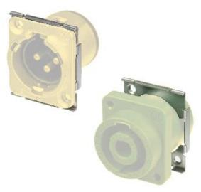
This fixing plate with M3 threads offers efficient and easy mounting of all D-sized panel connectors, without the need for nuts. It can be used with the connectors mounted front or rear of the panel by M3 screws.
