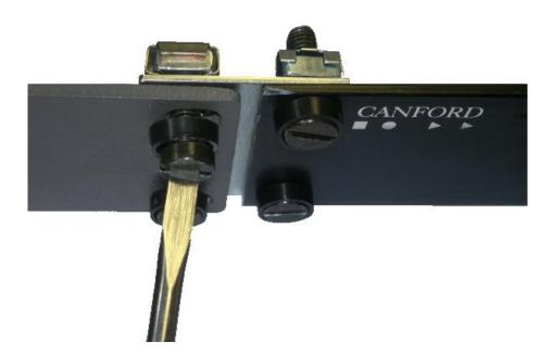
The joined panels can now be installed into a standard 19" width rack cabinet.
