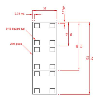
45-3360 CANFORD JOINING PLATE For half rack width panel, 1U 45-3361 CANFORD JOINING PLATE For half rack width panel, 2U
