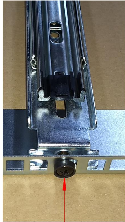
Rack screw secures bracket through front of mounting strip
