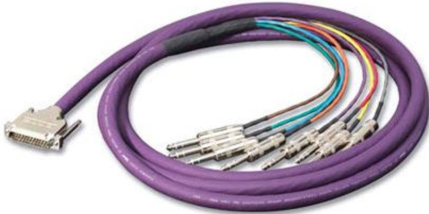
Suitable for Analogue audio input or output, (depending on if the D-sub is attached to an analogue input or output on the host device), this cable assembly is wired to the Tascam DTRS convention. Belden 7880A low-capacitance, individually screened, 110 Ohm eight-pair cable used. The D-sub 25-pin male connector has a metal-body and sensibly-sized thumb-screws.
