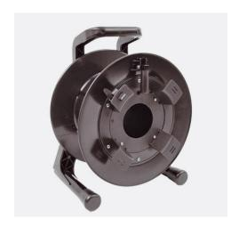
Black steel cable drum, with steel tube frame. Friction drum-brake incorporated into the frame to prevent movement in transit. Open hub plus four brackets on the flange face to enable the cable tail to be brought out from the hub of the drum at a gentle angle, (important for coaxial and essential for fibre cables), coiled and secured around the brackets. Folding winding-handle on the drum flange.
