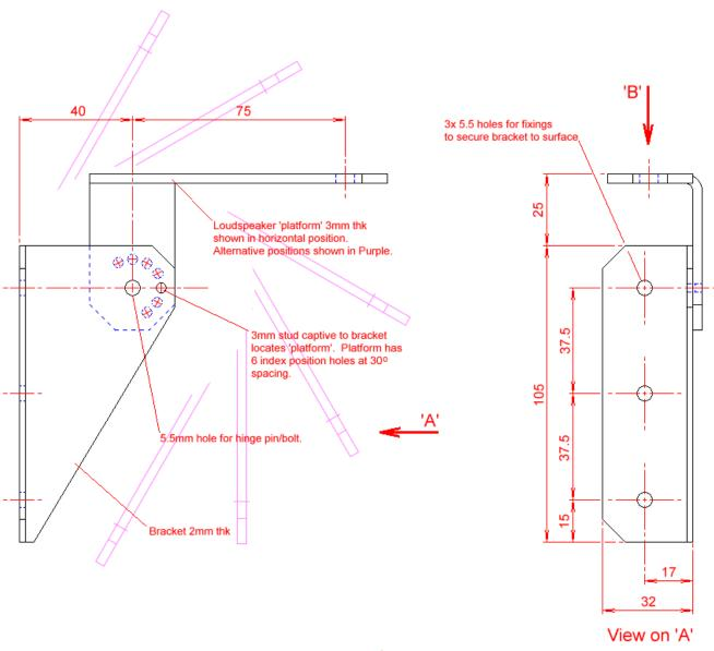
Assembly Drawing All dims in mm Not to scale
