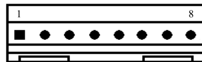
Connector viewed from component side
