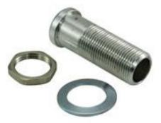
Flush bracket for mounting into work surfaces up to 45mm thickness. Requires 19mm mounting hole, supplied with fixing nut. Accepts 12.5mm spigot on both the standard and heavy duty adjustable mic arms. Plain aluminium finish.
