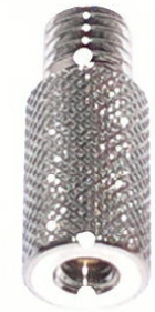
53-220 THREAD ADAPTER 375M-250F Overall: 31mm Male: 3/8" x 10mm Female: 1/4" x 15mm
