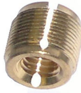
53-217 THREAD ADAPTER 625M-375F Overall: 14mm Male: 5/8" x 14mm Female: 3/8" x 14mm
