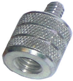
53-215 THREAD ADAPTER 250M-375F Overall: 27.5mm Male: 1/4" x 10mm Female: 3/8" x 10mm
