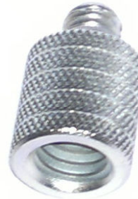
53-218 THREAD ADAPTER 375M-500F Overall: 30mm Male: 3/8" x 9.5mm Female: 1/2" x 12mm
