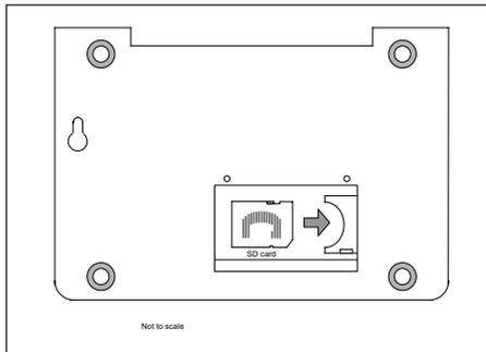
Insert the card oriented as shown (pins away from you), and slide into the card holder as far as it will go.
