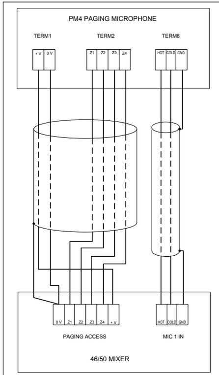
Note in this example that as Zones 5-16 are not in use, no connections need to be made to Z5-Z8 on TERM2, or to Z9-Z16 on TERM4.
