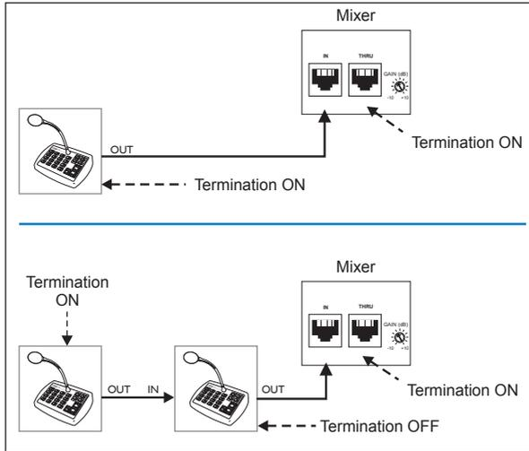
The termination is set in the PM with jumper J4. See “PCB layout diagrams” on page 52 for jumper locations. The factory default setting is for the termination to be set ON. If the PM being configured is ‘mid-chain’, with both its CAN PORT IN and CAN PORT OUT connectors in use, set the termination to OFF by removing the jumper.
