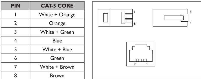
The IN port will only be used when the system has more than one PM. To interconnect two PMs, connect the OUT port of one to the IN port of the next 'in the chain' using the same wiring standard as shown in the table above. See "Systems with multiple paging microphones" on page 47 for full details.
