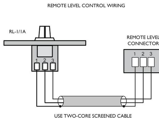
Maximum reliable cable run is 100 m. An RL-1 will control the level in the channel from zero ("off") to the maximum determined by the setting of the rear panel **LEVEL** preset control.
