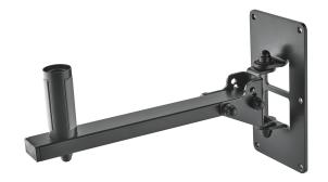
Robust wall mount for holding speakers with flange socket up to 25 kg. The swivel range is continuously adjustable up to 120°. The tilt can be fixed in three steps with 0°, -12.5° and -25°. A patented expanding mandrel ensures a wobble- and vibration-free fit of the speaker. The solid steel construction and durable powder coating ensure long-lasting use.
