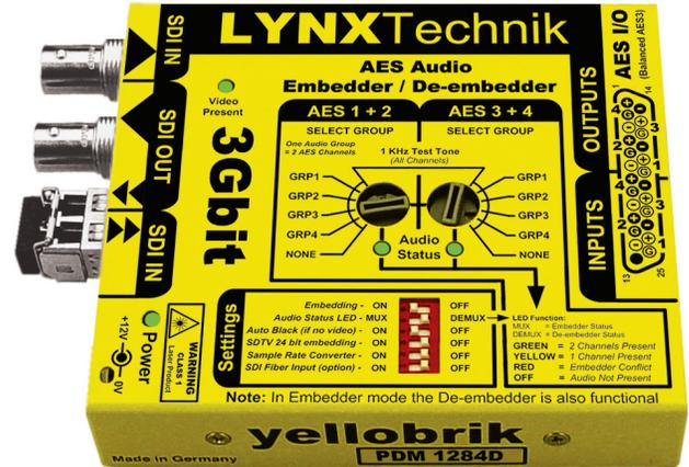
The PDM 1284 D is a versatile AES audio embedder and de-embedder designed for a wide range of SDI video formats up to 3Gbit. It supports balanced AES3 audio I/O using a 25 pin SubD connector.
