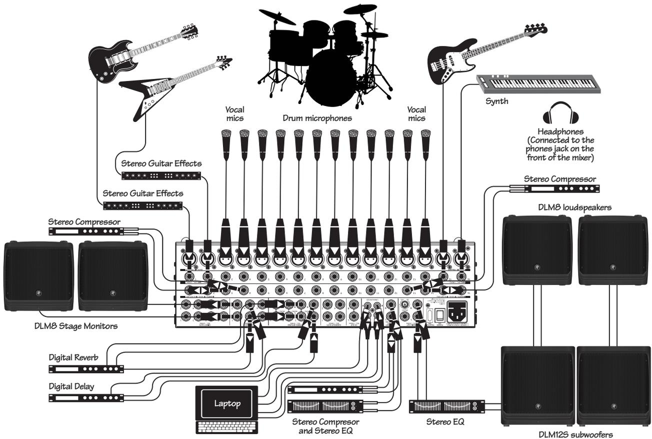
The rhythm and lead guitars play through stereo effects processors plugged into the line inputs of channels 1 and 2. Microphones are connected to the mic inputs of channels 3-14 with vocal compressors connected to the channel 3-4 and 13-14 insert jacks. [Drums are mic'd on channels 5-12]. A bass guitar is connected to the line input of channel 15, while a synth is connected to the line input of channel 16.
