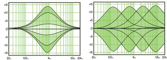
Most of the root and lower harmonics that define a sound are located in the 100 Hz–8 kHz frequency range, and you can create drastic changes with these two knobs. Many engineers use mid EQ to cut midrange frequencies, not boost them. One popular trick is to set the mid fully up, turn the frequency knob until you find a point where it sounds just terrible, then back the mid down into the cut range, causing those terrible frequencies to disappear. Sounds silly, but it works. Sometimes.
