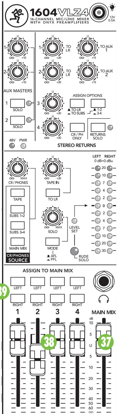
mix, engage both the assign to main mix, left and right switches. The signal will be sent to both sides, and will be attenuated just enough to preserve constant loudness, just like the channel pan [31] knobs when set in the center.
