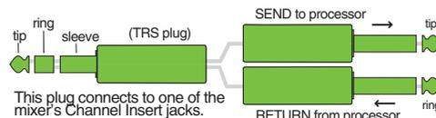
Even though channels 1–8 already have direct out [5] jacks, insert jacks can also be used as channel direct outputs; post-gain, pre-low cut, and pre-EQ. See the connector section on page 29 showing three ways to use insert cables.
