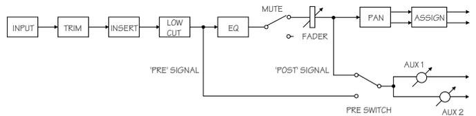
In post mode (switch up), aux 1 and 2 will follow the EQ [32], low cut [33], fader [25], and mute [30] settings. If you fade the channel, you fade the send. This is a must for effects sends, since you want the levels of your "wet" signals to follow the level of the "dry."
