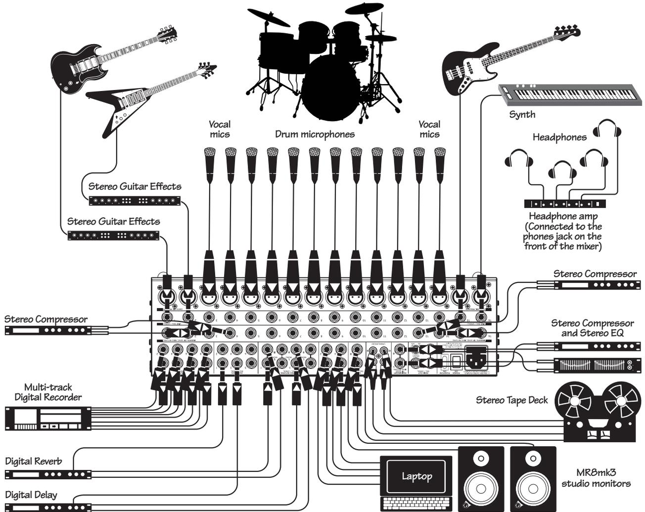
The rhythm and lead guitars play through stereo effects processors plugged into the line inputs of channels 1 and 2. Microphones are connected to the mic inputs of channels 3-14 with vocal compressors connected to the channel 3-4 and 13-14 insert jacks. [Drums are mic'd on channels 5-12]. A bass guitar is connected to the line input of channel 15, while a synth is connected to the line input of channel 16.
