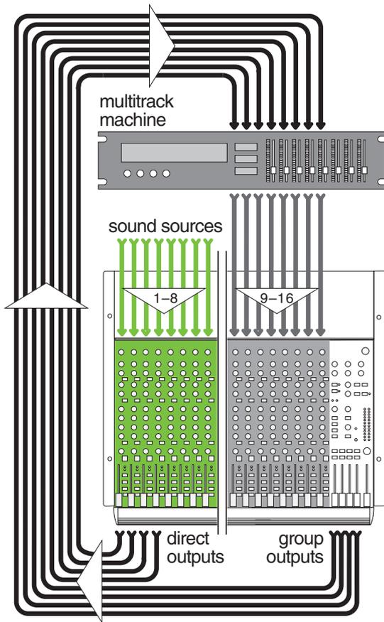
The outputs of the multitrack are then patched to the next eight line [2] inputs on the 1604VLZ4 (multitrack out 1 to line input 9, 2 to 10, 3 to 11, etc.). These channels (9–16) will be assigned to the mixer’s output section, delivering the signals to their ultimate destination, which may be your mixdown 2-track, your control room system, or your headphones.
