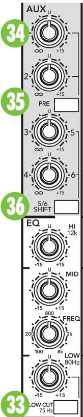
These four knobs tap a portion of each channel's signal, mix them together and send them to the aux send [6] outputs. They are off when turned fully down, deliver unity gain at the center detent, and can provide up to 15 dB of gain turned fully up. Chances are you'll never need this extra gain, but it's nice to know it's there if you do.
