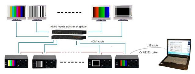
The HDMI 2.0/3G-SDI Signal Generator is intended to be used to test HDMI sink devices, which may include HDMI or SDI matrix, switches, Switchers, splitters, TV sets, etc.
