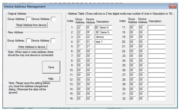
The Signal Generator can be used to set up a large test system. All Signal Generators and Signal Analyzers in a system can be cascaded by using the RS232 (3 pin) Phoenix connector. When more than one Signal Generator is connected on a single serial chain (Bus), these devices must have unique (different) identification address.
