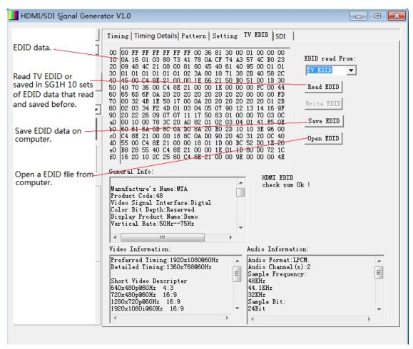
**Note:** The Signal Generator can save 10 sets of EDID data. This function is useful when the installer is in the field analyzing HDMI system problems.
