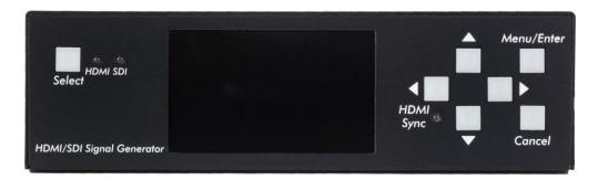
For SDI applications: Follow the same procedure as above, but select SDI mode, use SDI coax cable of appropriate grade, and ensure that the SDI Out LED is On. If this LED is Off, but the HDMI Out LED is On, then press the 'Select' button to change to SDI mode.
