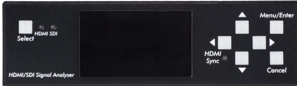
For SDI applications, follow the same method to set up the system. But you need to ensure the SDI OUT LED is lit (is on). If this LED is off but HDMI LED is on, then press the button to change the mode to SDI mode.
