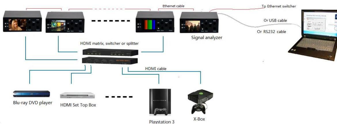
The HDMI 2.0/3G-SDI Signal Analyzer is an SDI receiver or HDMI® sink emulator that can be used to test SDI or HDMI Sources, such as Media Players, BD players, Matrix Switches, Switchers, Splitters, Repeaters, and numerous other HDMI devices for proper functionality.
