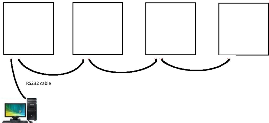
5. Set different Serial address for each Signal Analyzer and Signal Generator (if any).
