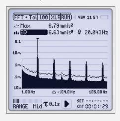
The Vibration Option turns the XL2 into a flexible vibration meter, with FFT analysis and data logqing, for frequencies down to 0.7 Hz.
