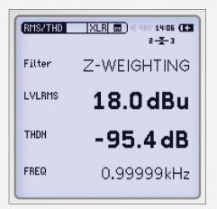
With a balanced XLR and unbalanced RCA input, the XL2 is a high-performance audio analyzer. It simultaneously measures balance, RMS level, frequency, and harmonic distortion (THD + N).
