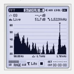
The real-time FFT is the ideal tool for detecting comb filters and resonant frequencies. The XL2 measures the actual level and the time-averaged Leq level in three frequency ranges.
