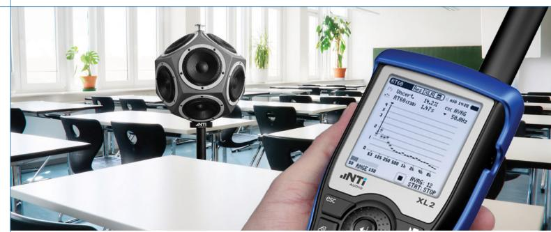
The standard XL2 contains all the necessary functions for measuring room and building acoustics, including reverberation time in octave bands. An intelligent auto-naming process helps with the assignment of each result as a sending/receiving room or ambient level measurement.
