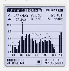
Real-time analysis RTA is an ideal tool for optimizing sound systems. In addition to the broadband levels, the XL2 simultaneously measures the real-time spectrum in 1/3 or 1/1 octave band resolution.
