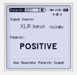
Other measurement functions determine the speaker polarity, help with the setup of delay lines or represent the signal in an auto-ranging oscilloscope.
