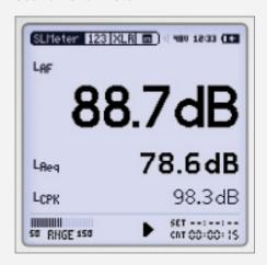
The XL2 with measurement microphone is a precise Sound Level Meter. All measurement results are available simultaneously, e.g. Leq, Lmin, Lmax, and LCpeak, with the frequency weighting A, C, Z and the time weighting Fast, Slow and optional Impulse.
