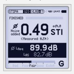
The XL2 measures STI and CIS values for speech intelligibility of evacuation and announcement systems in accordance with the IEC 60268-16 and DIN VDE 0833-4 standards. A correction of the determined speech intelligibility by the addition of the spectrum of the ambient noise is possible.
