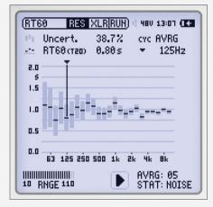
Measure the reverberation time in a room with automatic triggering from an impulse or gated pink noise sound source.
