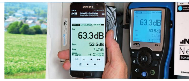
The XL2 Sound Level Meter provides all the functions needed to measure and monitor noise. Its removable SD card offers plenty of space to record levels, spectra and audio files. The data can also be read out during an ongoing measurement via its USB interface.
