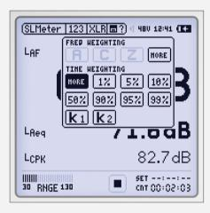
The Extended Acoustic Pack Option provides advanced acoustic measurement possibilities. The option enables the recording of linear wav files, percentile statistics, sound exposure levels, spectral logging in 100 ms intervals, RT60 in 1/3 octave resolution, event monitoring, and much more.
