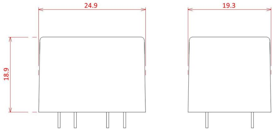
Suitable for line level input stages using the current mode or 'zero field' technique. This removes most of the artefacts normally associated with audio transformers whilst retaining the desirable galvanic isolation RFI blocking.
