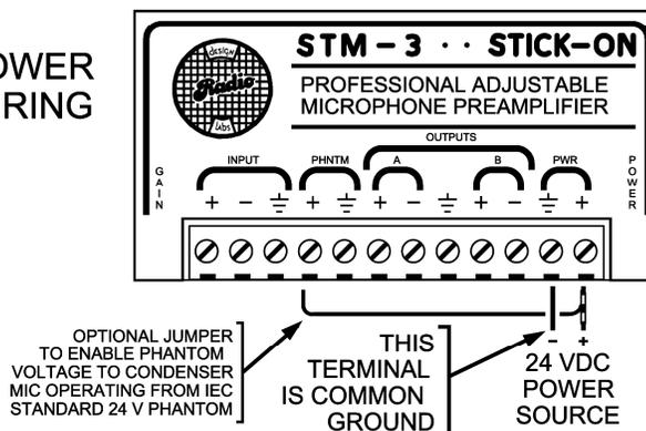
NOTE: THE STM-3 WILL OPERATE (WITH REDUCED HEADROOM) ON SUPPLY VOLTAGES FROM 9 TO 23 VDC.
