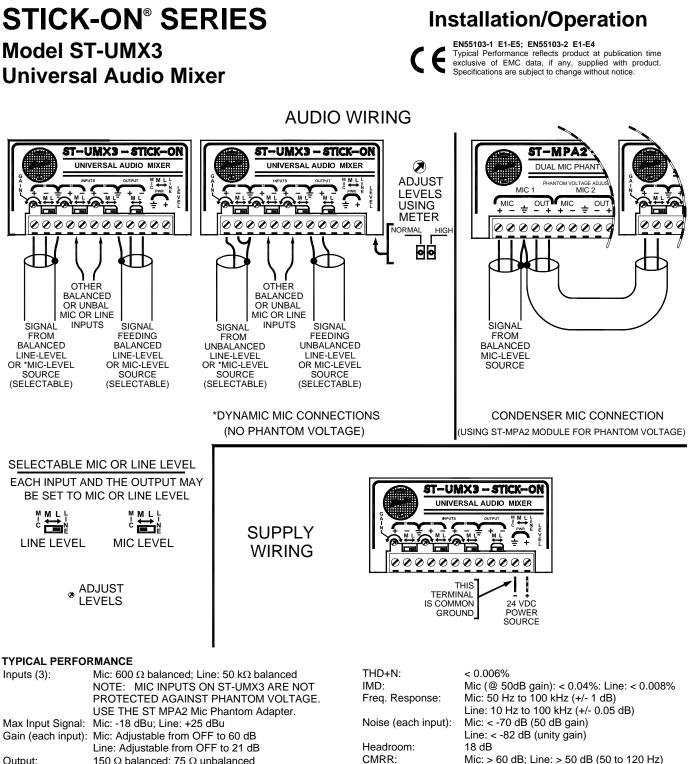
150  $\Omega$  balanced; 75  $\Omega$  unbalanced Output: Output Signal: +4 dBu nominal, mic level 50 dB below line level
