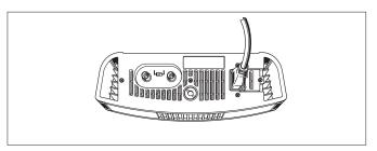
Install the SZI 1029 high power radiator in a vertical (or almost vertical) position. The cables are guided downwards.
