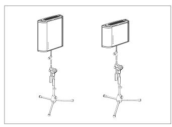
The SZI 1029 high power radiator is provided with an interchangeable thread for mounting it to stands with 3/8" or 1/2 "threads using an adaptor (included in the scope of delivery).
