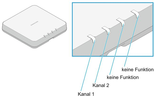
When the LEDs are displaying the status of the entire device and not the individual channels, all four LEDs (SL MCR 4 DW variant) or the first two LEDs (SL MCR 2 DW variant) will light up or flash.
