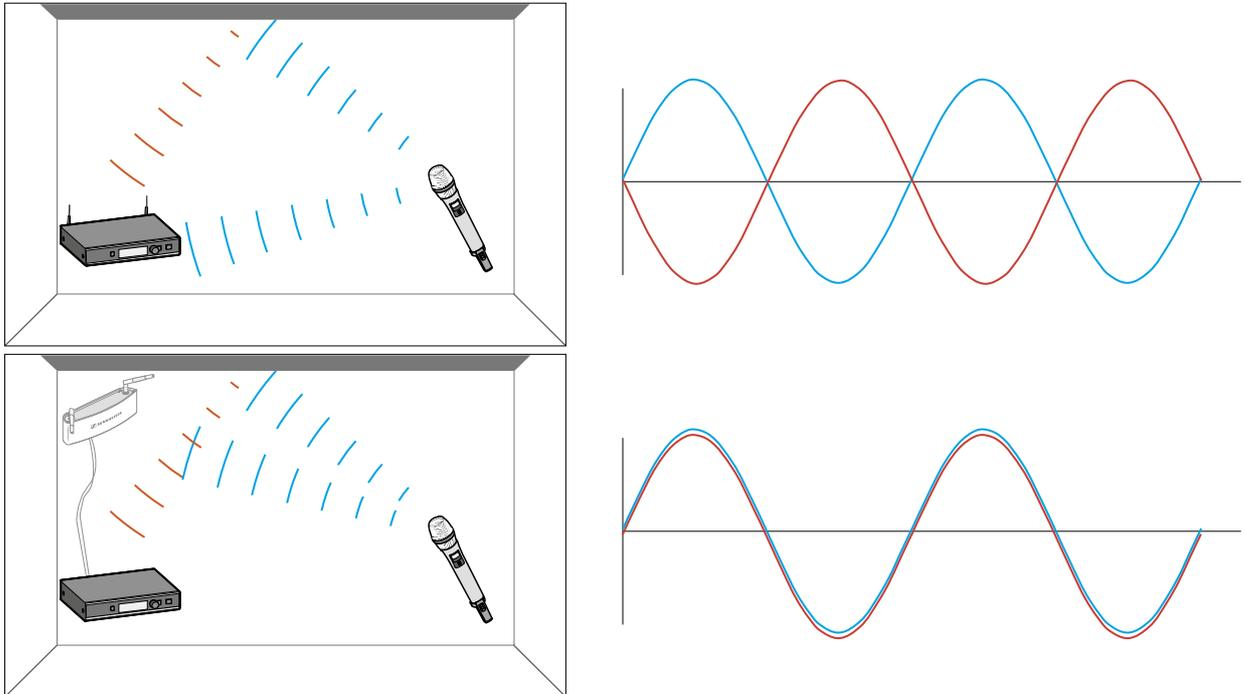
The signal is reflected by the electrically conducting surface. At worst, the blue signal and the red reflected signal are out of phase when they reach the receiver so that the two signals cancel each other out.
