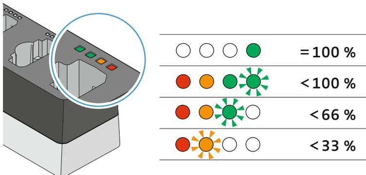
Details: „Meaning of the charging slot status LEDs“
