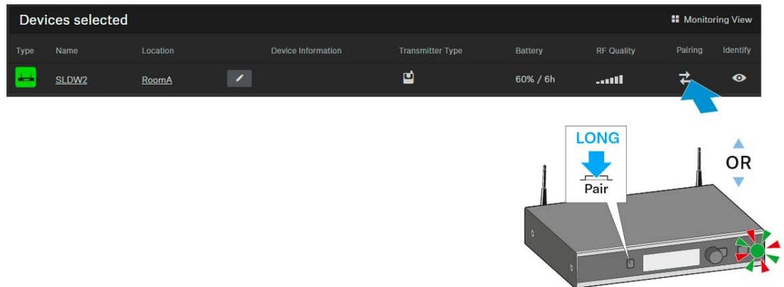
First, **Identify** appears on the display panel of the receiver. The **Pairing** message then appears.
