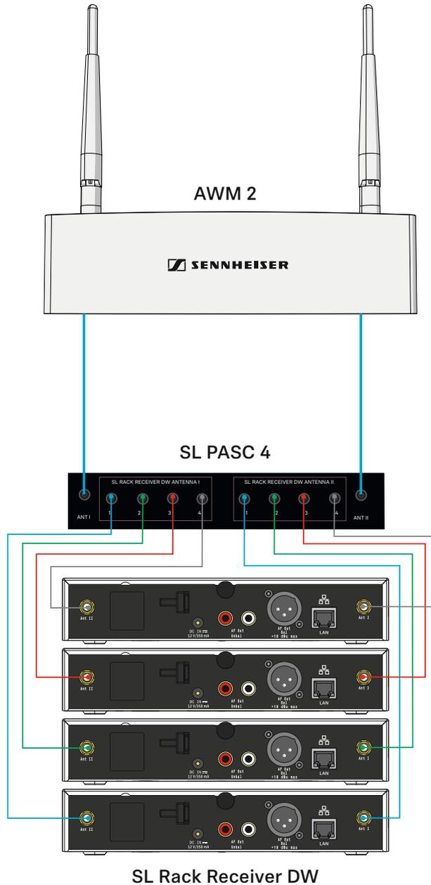
Use the following Sennheiser cables for connecting the AWM 2 to the SL PASC 4:
