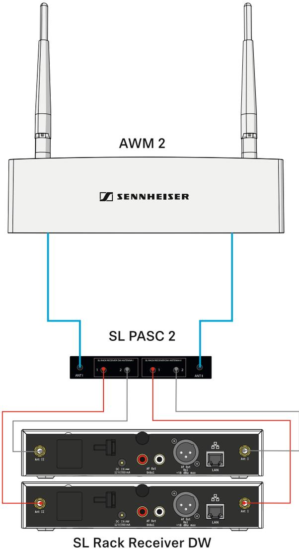
Use the following Sennheiser cables for connecting the AWM 2 to the SL PASC 2:
