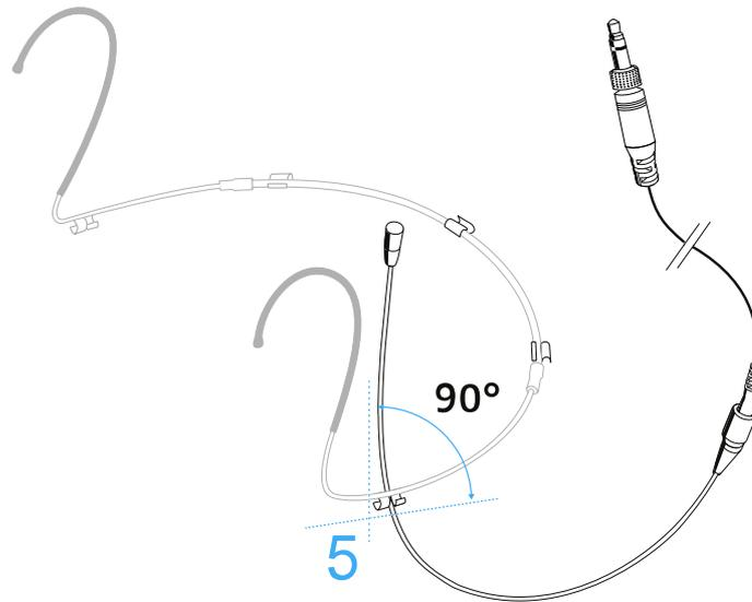
▷ Press the microphone boom into the two clips **3** and **4**.
