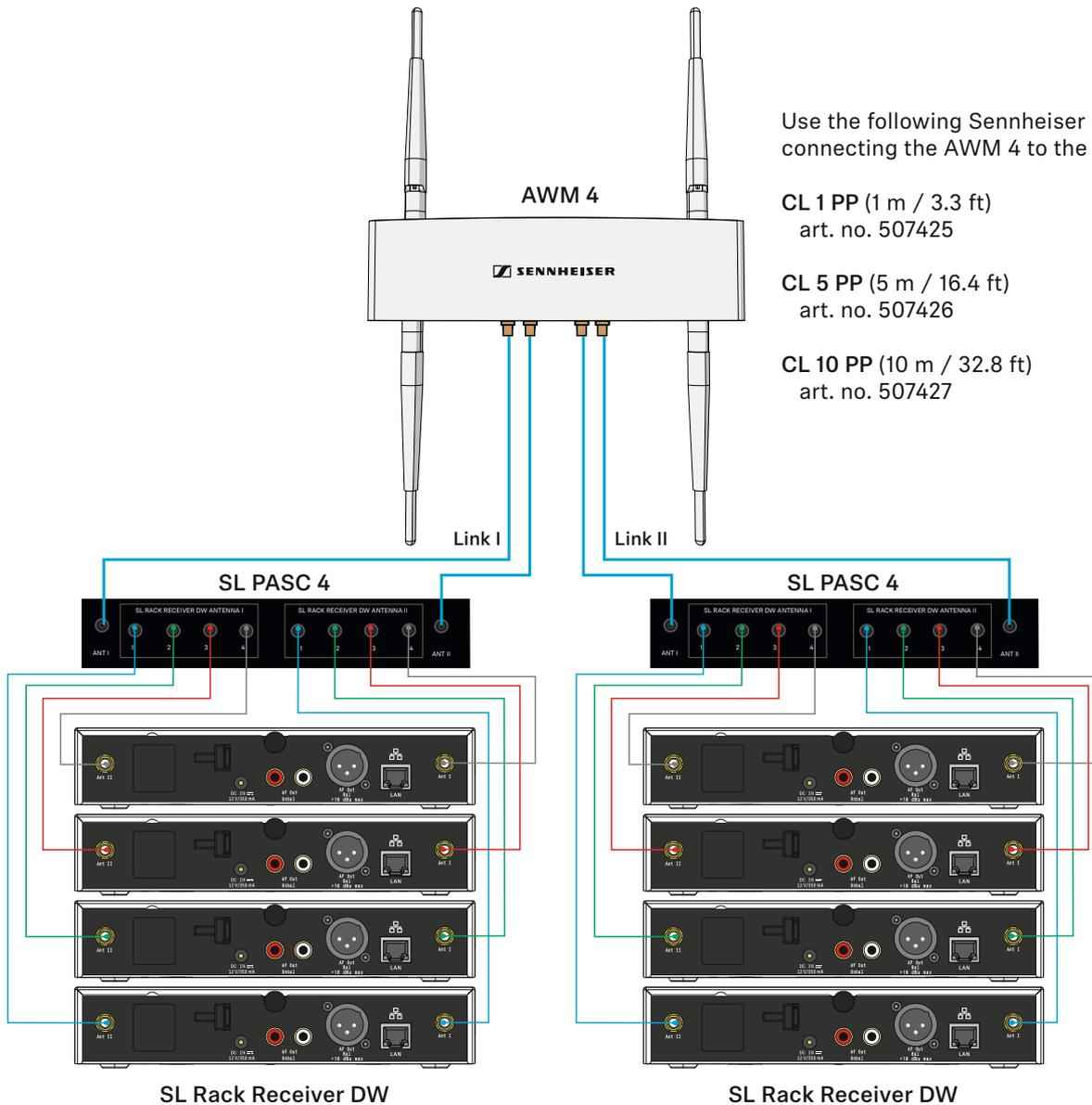
Use the following Sennheiser cables for connecting the AWM 4 to the SL PASC 4:
