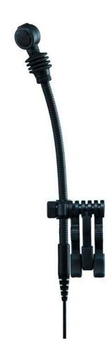
The e 608 has a newly developed clamp and gooseneck mounting, which enables the capsule to be positioned close to the signal source for high realism and high level output. Extensive damping and shock mounting isolates the capsule and signal from extraneous vibration, noise and impact.
