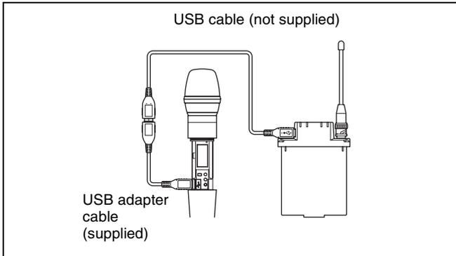
*For details on receiver operations, refer to the operating instructions supplied with the receiver.*
