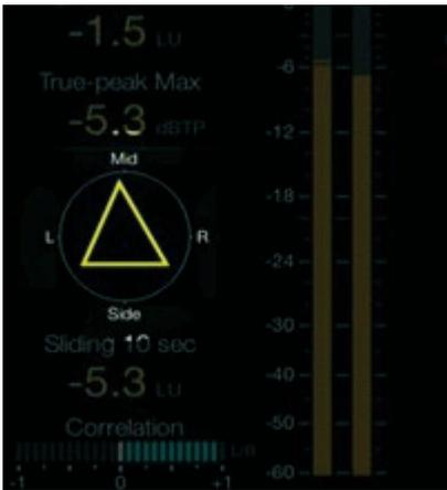
The top of the triangle will point toward the top/center of the semi circle when a perfect left-right balance is achieved. The width is indicated by how broad the base of the triangle is.
