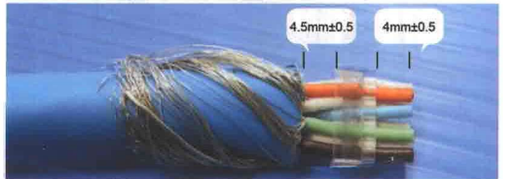
6. Slide into insert and trim
