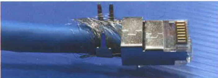
7. Slide assembly into plug body
