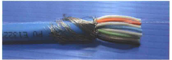
4. Cut off the foil and twist drain wire
