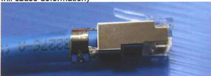
11. Cut the remaining drain wire
