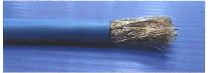
2. Strip 20mm sheath from the cable
