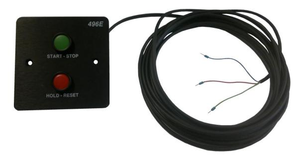
The 496E stopwatch control unit is intended for manual operation. Facilities are provided for start/stop display, hold or 'freeze' and reset operations. The start/stop control may be used for single event timing either on a continuous or interrupted basis. The display hold control permits the recording of a series of sequential times. Alternate switch activations stop and restart the display while the internal counter continues operation.
