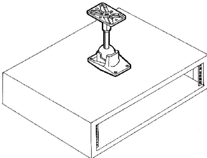
Ceiling mounting arrangement using Omnimount 100STX-MP (stock code 18-588, not included with pod)
