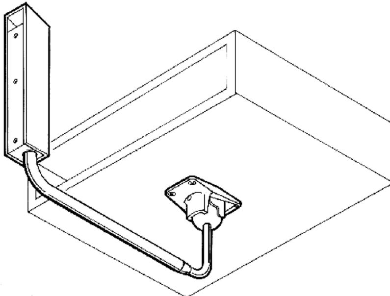
Wall mounting arrangement using Omnimount bracket 100WBX (stock code 18-576, not included with pod)
