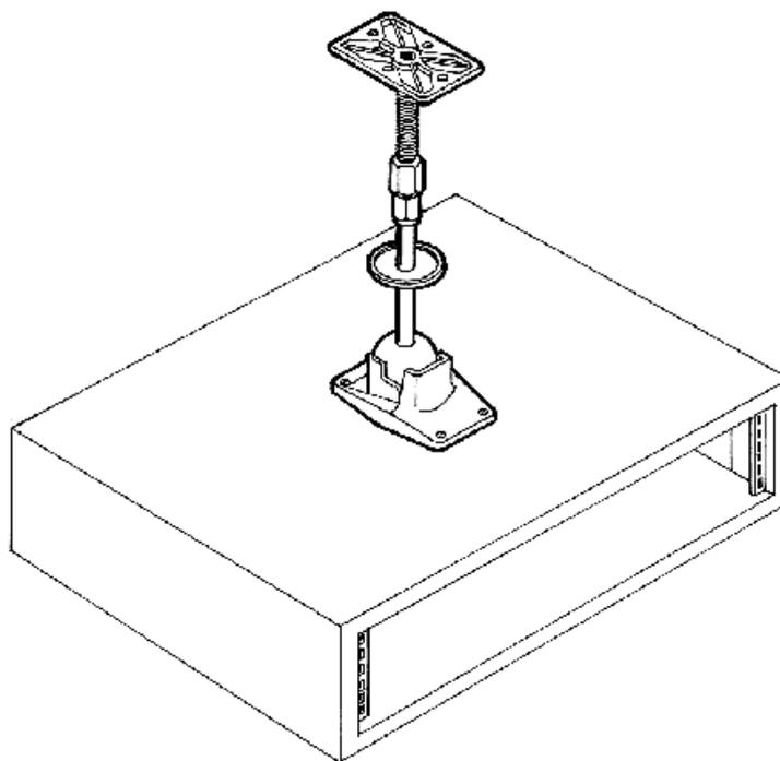
Ceiling Mount arrangement where suspension from a high ceiling or through false ceiling is required, using Omnimount parts:
