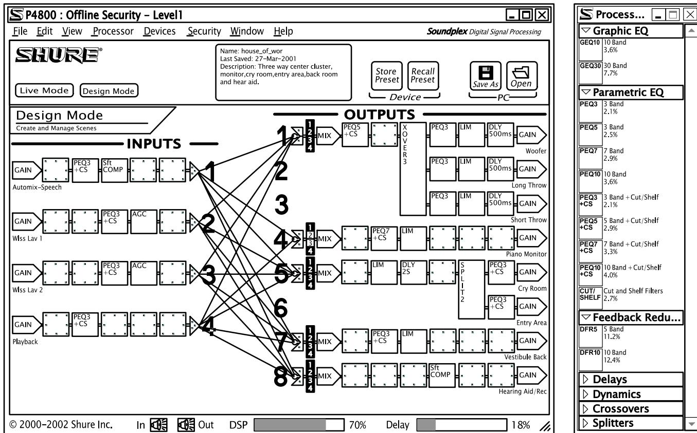
The primary interface for the P4800 is a Windows-based software program that mimics the functional block diagrams used in sound system design. Unlike many other DSP products that constrict design freedom with preset templates, the processing blocks in the P4800 can be applied in any order, to any input or output. Processing blocks can be copied and pasted to duplicate processors across multiple channels. They can also be linked for more efficient stereo or global control.
